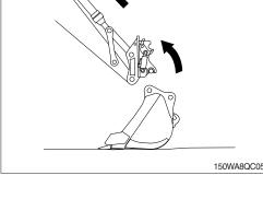
(10) To engage the quick coupler, release the quick coupler button on the right RCV lever.
