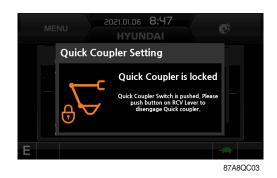
(5) To unlock the quick coupler, press the quick coupler button on the right RCV lever.To maintain the unlock status of the quick coupler the operator must maintain pressing the coupler button.
